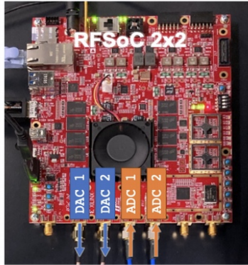
Readout system with RFSoc (FPGA+CPU+ADC+DAC) (Kyoto、Tohoku)
